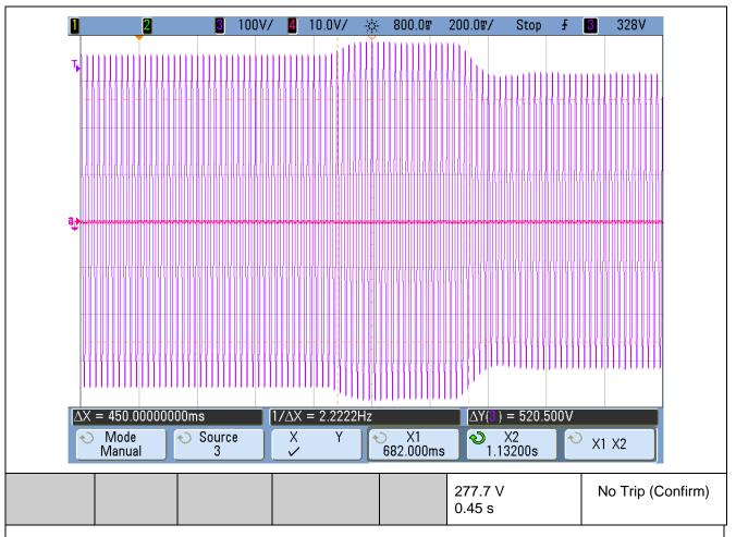
Note for Voltage tests the Voltage required to trip is the setting  $\pm 3.45$  V. The time delay can be measured at a larger deviation than the minimum required to operate the protection. The No trip tests need to be carried out at the setting  $\pm 4$  V and for the relevant times as shown in the table above to ensure that the protection will not trip in error.
